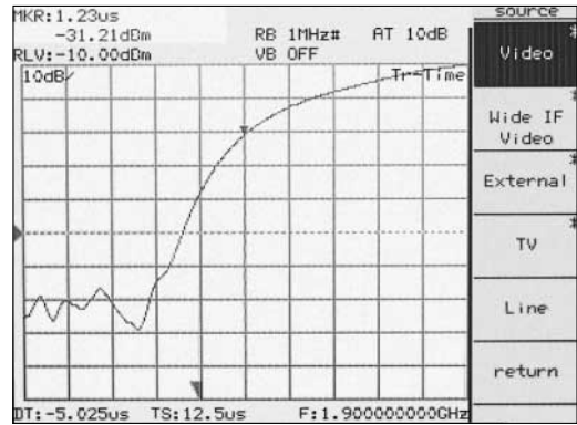
High-speed time domain measurement (TS = 12.5 \mu s)
